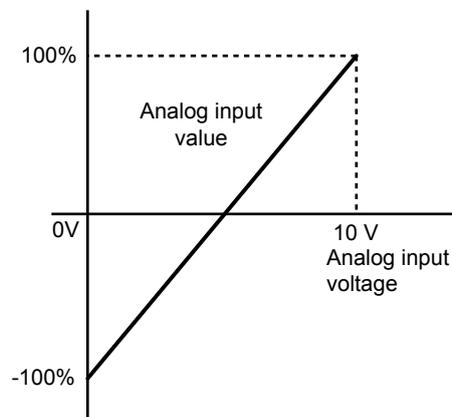
Figure 5.65 Analog Input without Limit (Bias Setting -100%)
