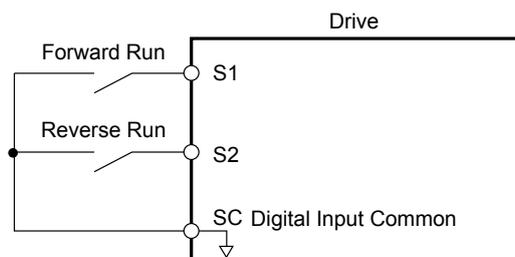
Figure 5.50 Example Wiring Diagram for 2-Wire Sequence
