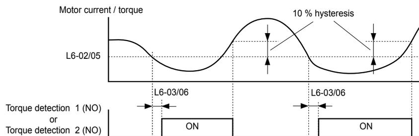
**Figure 5.86 Undertorque Detection Operation**
