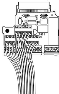
Figure 7.8 Removable Terminal Board disconnected from the drive
