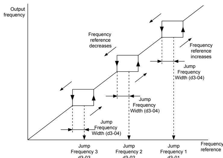
Figure 5.32 Jump Frequency Operation
