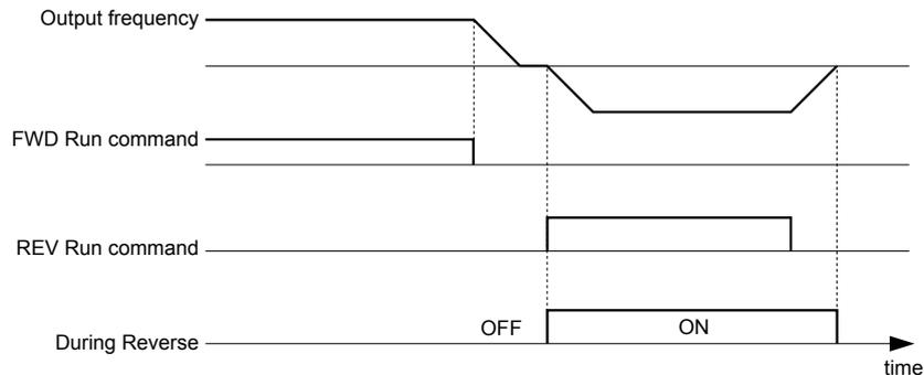
Figure 5.62 Reverse Direction Output Example Time Chart
