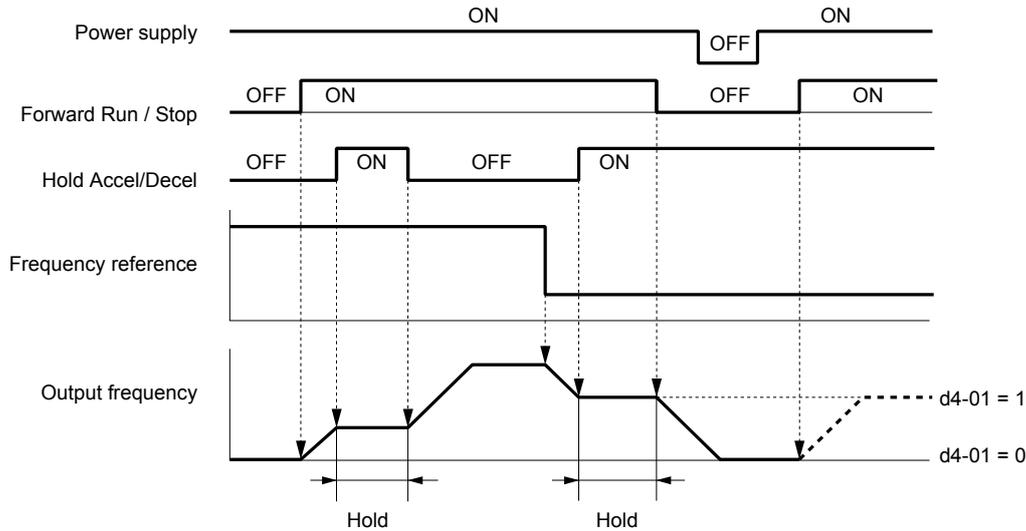
Figure 5.33 Frequency Reference Hold with Accel/Decel Hold Function
