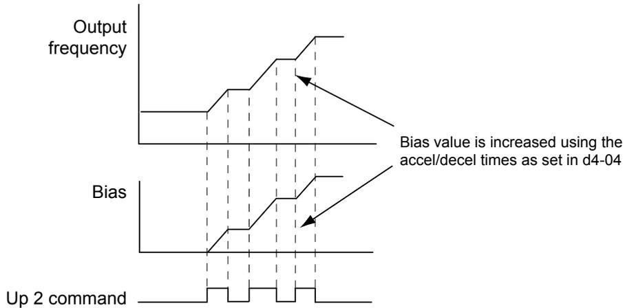
Figure 5.36 Up/Down 2 Bias when d4-03 = 0.0 Hz
