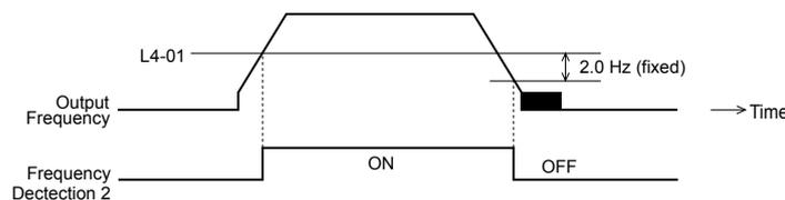
Figure 5.83 Frequency Detection 2
