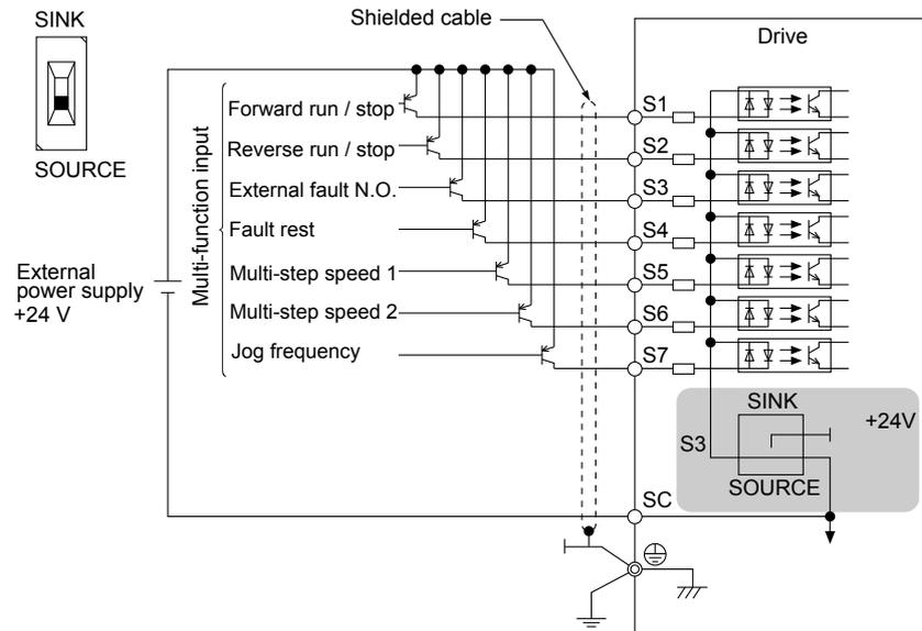
Figure 3.23 Source Mode: Sequence from PNP Transistor (+24 V Common)
