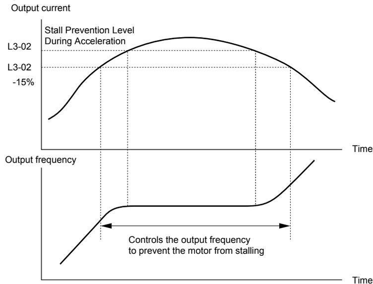
Figure 5.78 Stall Prevention During Acceleration for Induction Motors
