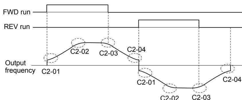
Figure 5.24 S-Curve Timing Diagram - FWD/REV Operation
