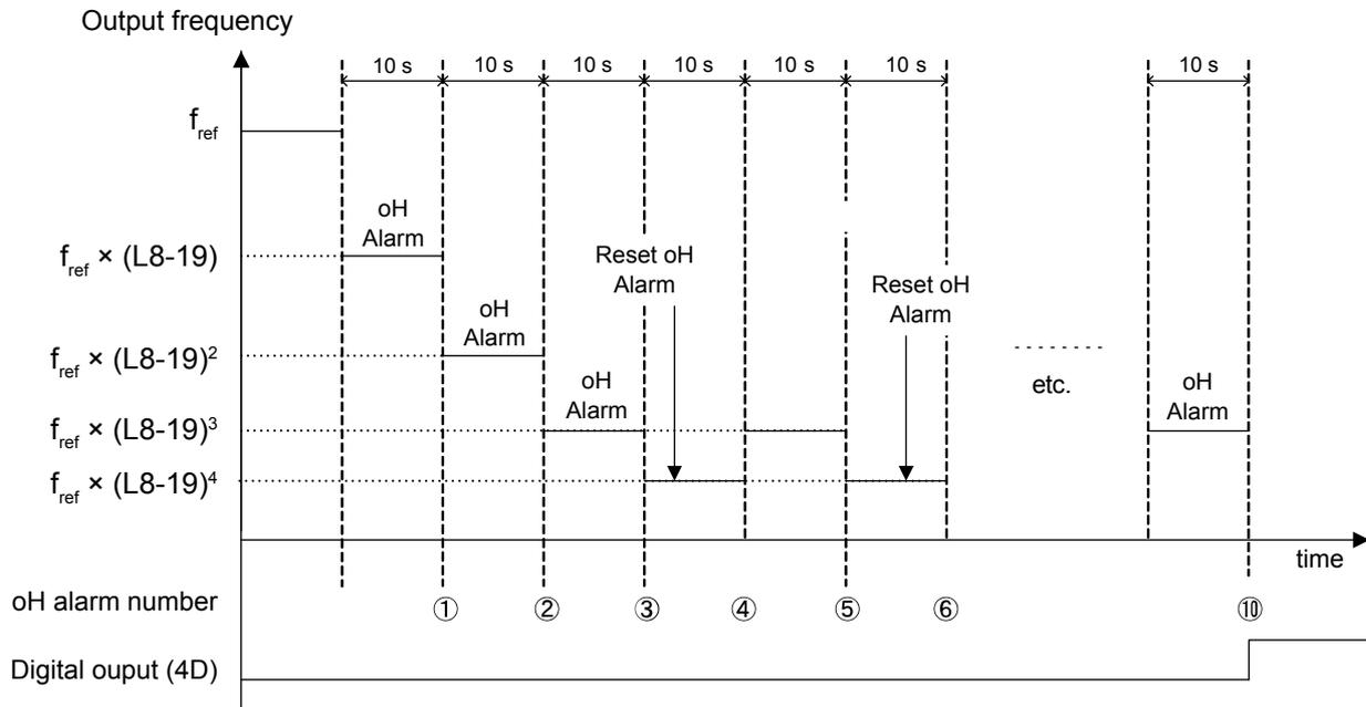
Figure 5.87 Output Frequency Reduction During Overheat Alarm
