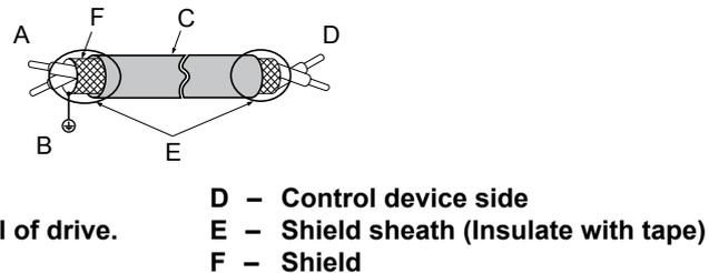
Figure 3.19 Preparing the Ends of Shielded Cables
