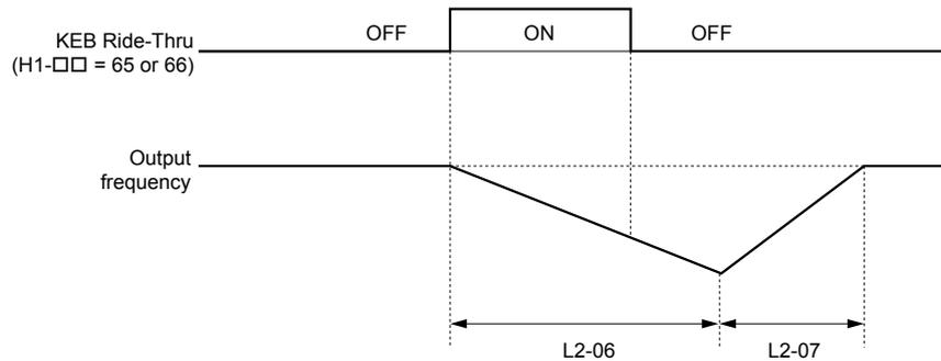
Figure 5.76 KEB Ride-Thru Timing Diagram for Multiple Drives
