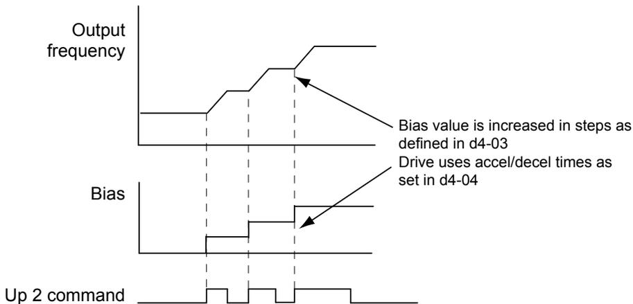
Figure 5.37 Up/Down 2 Bias when d4-03 > 0.0 Hz
