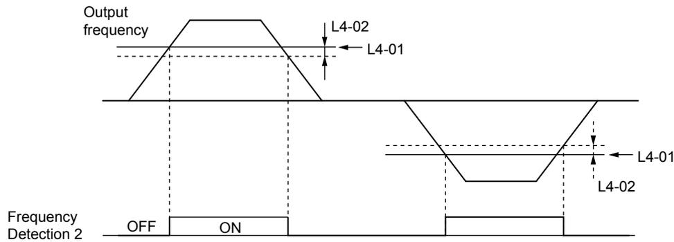
Figure 5.57 Frequency Detection 2 Time Chart
