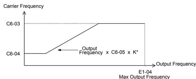
Figure 5.28 Carrier Frequency Changes Relative to Output Frequency
