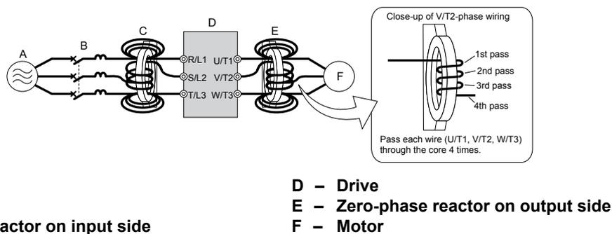
Figure 8.10 Zero-Phase Reactor
