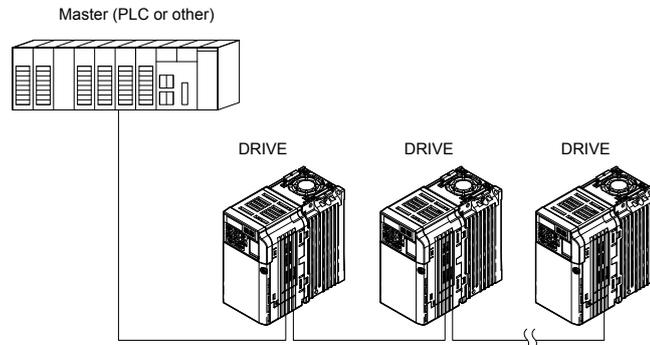
Figure C.1 Connecting Multiple Drives to a PLC
