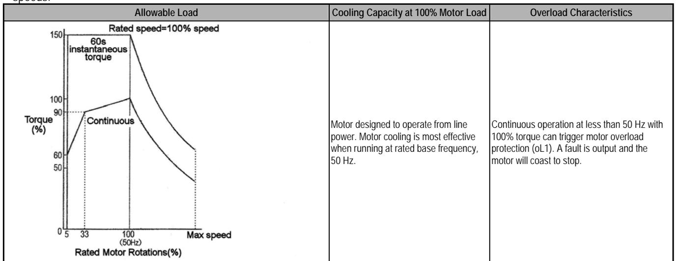
**Note:** Select a method to protect the motor from overheat by setting L1-01 between 1 and 4 or 6 when running a single motor from the drive. An external thermal relay is not needed.
