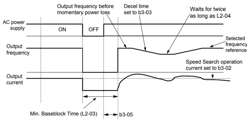
Figure 5.13 Current Detection Speed Search after Power Loss
