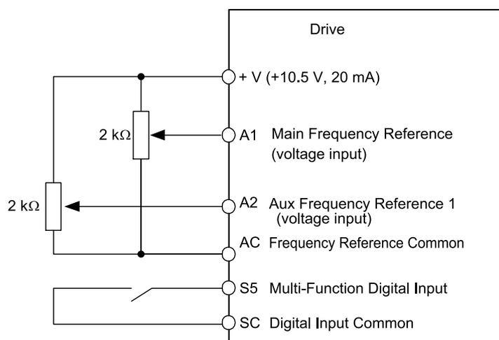
Figure 5.3 Switching between Analog Reference 1 and 2
