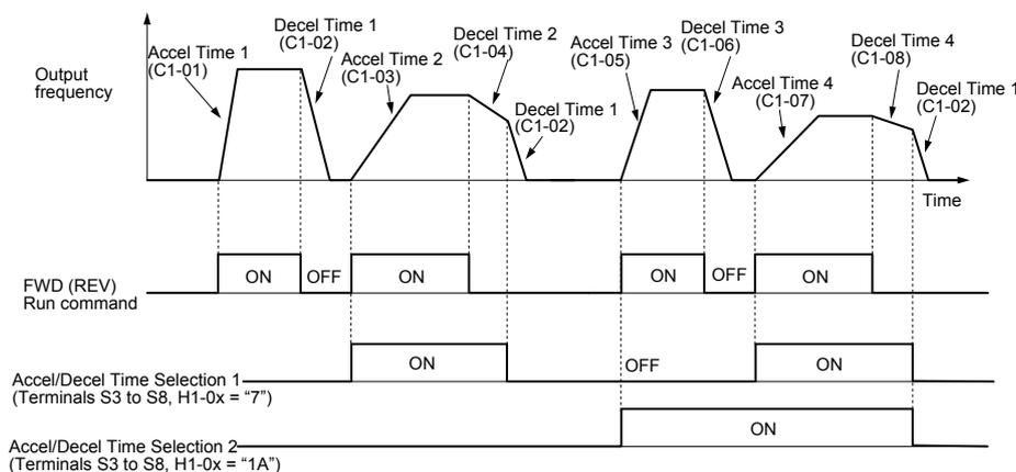
Figure 5.22 Timing Diagram of Accel/Decel Time Change
