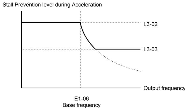
Figure 5.80 Stall Prevention Level and Limit During Acceleration
