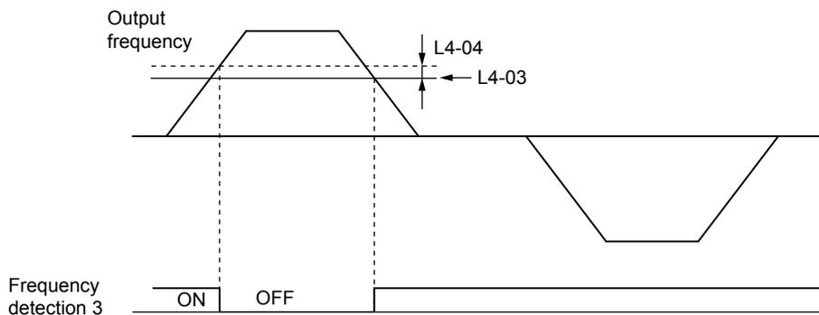
Figure 5.60 Frequency Detection 3 Example with Positive L3-04 Value
