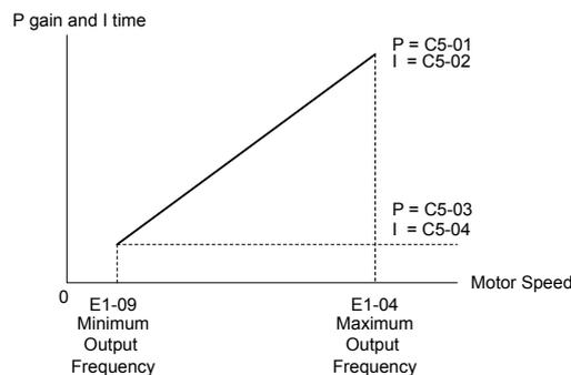
**Figure 5.27** Adjusting ASR Proportional Gain and Integral Time
