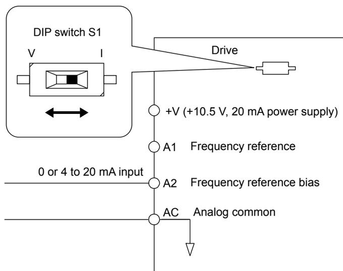
Figure 5.2 Setting the Frequency Reference by Current Input
