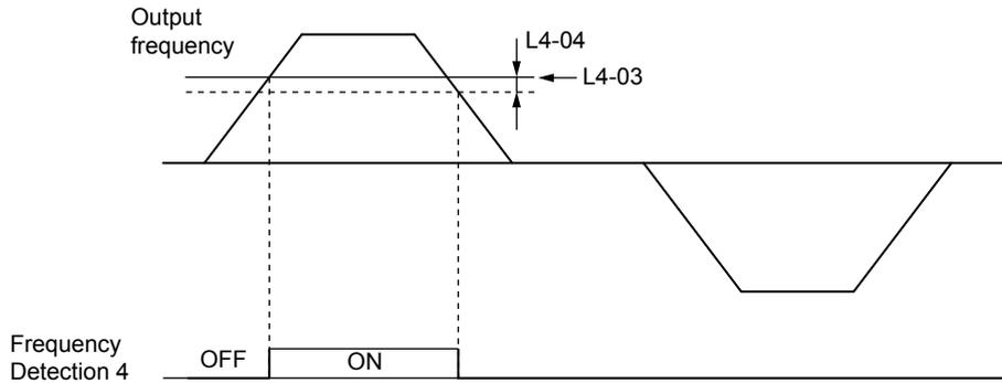
Figure 5.61 Frequency Detection 4 Example with Positive L3-04 Value
