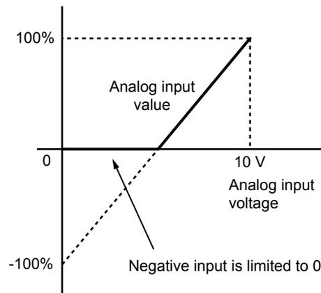
Figure 5.64 Analog Input with Limit (Bias Setting -100%)
