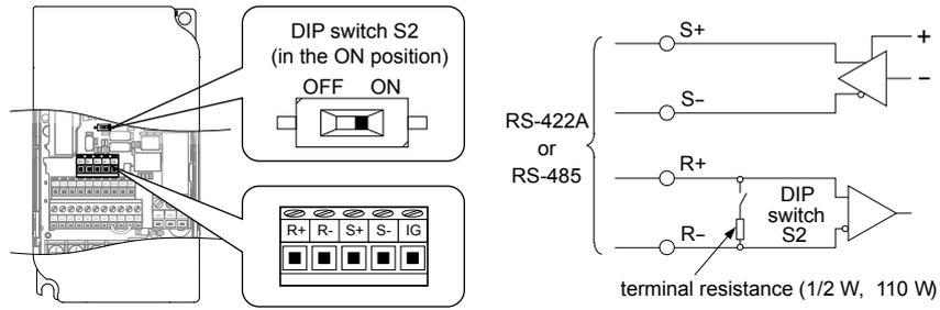
Figure C.5 Serial Communications Terminal and DIP Switch S2
