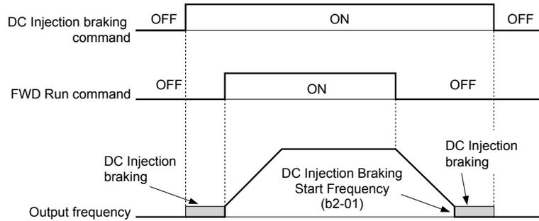
Figure 5.51 DC Injection Braking Input Timing Diagram
