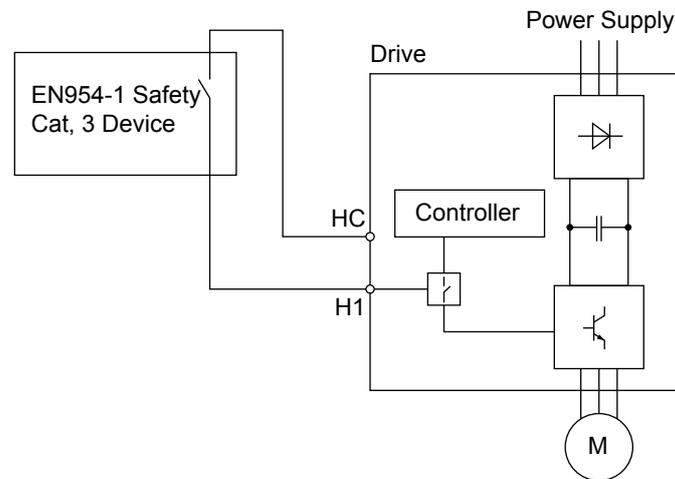
Figure D.9 Safe Disable Wiring Example
