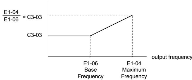
Figure 5.25 Slip Compensation Limit
