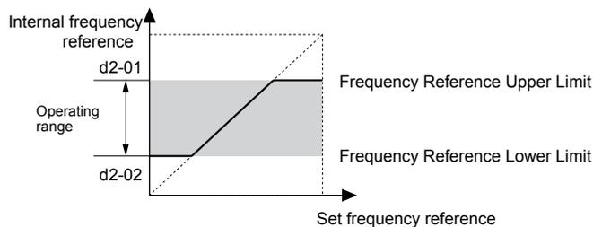
Figure 5.31 Frequency Reference: Upper and Lower Limits
