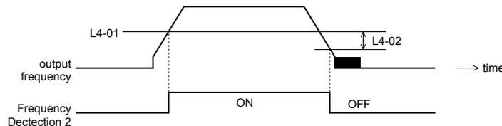
Figure 4.10 Frequency Detection 2
