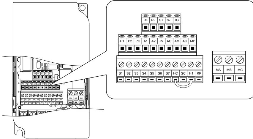
Figure 3.16 Removable Control Circuit Terminal Block (CIMR-VA□□□□□□□□; CIMR-VU□□□□□□□□)
