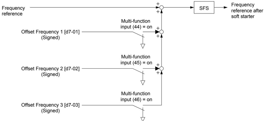
Figure 5.38 Offset Frequency Operation
